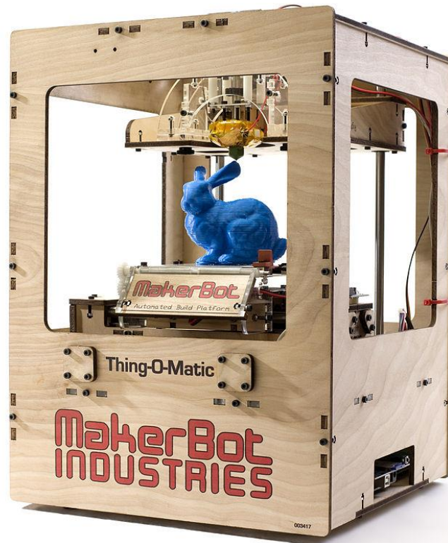
Impressora Makerbot® Thing-O-Matic. Extret de: https://en.wikipedia.org/wiki/MakerBot
