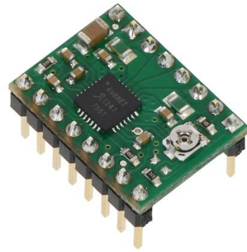
Driver Pololu A4988. Extret de: https://www.pololu.com/product/1182/pictures#lightbox-picture0J4578
