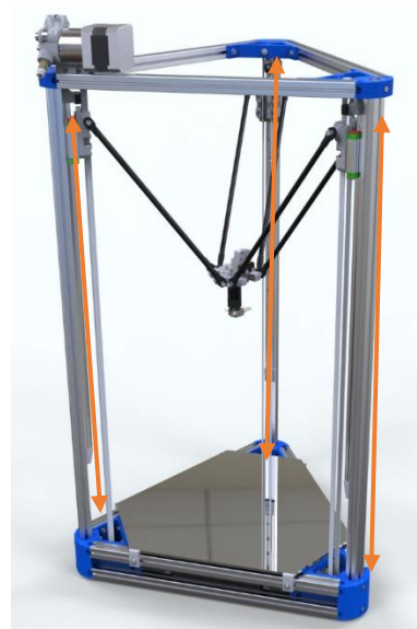
Eixos del moviment en una impressora Delta. Extret de: https://grabcad.com/library/kossel-delta-configuration-3d-printer-1
