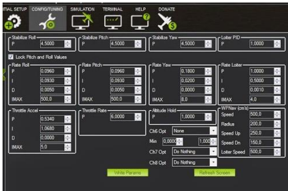
Fig 3.8 Finestra de valors PID a Mission Planner
